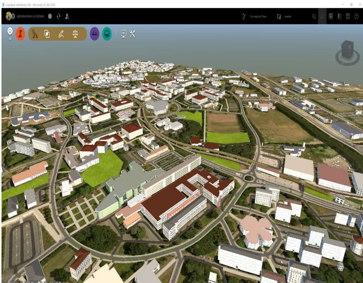
Figure 9.b. SUNRISE project Using the base map of OSM and provides a 3D City Model with LoD2 - the smart campus at the University of Lille, this model has been prepared by with Autodesk InfraWorks 360
